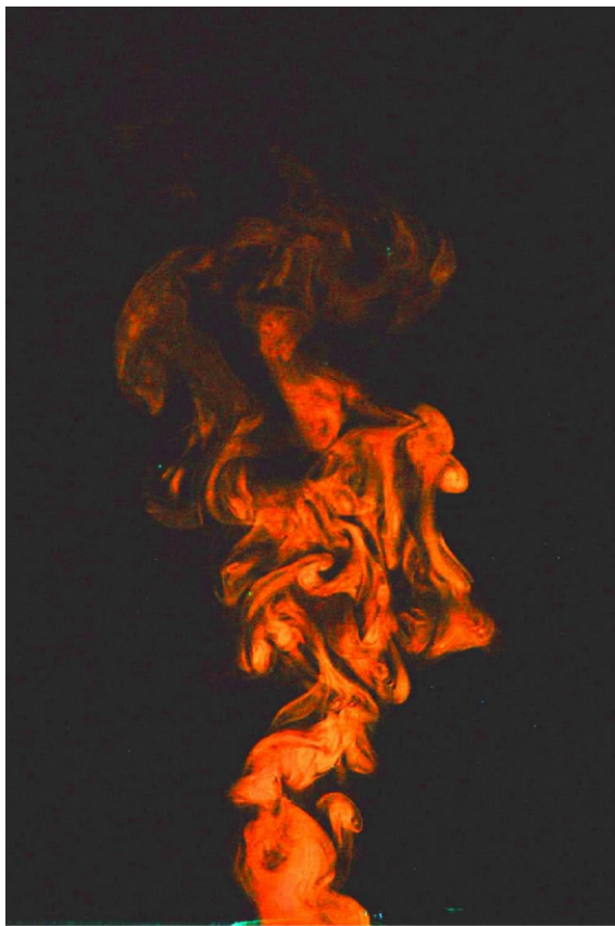
Fig. 7. Structure of turbulent buoyant plume.
